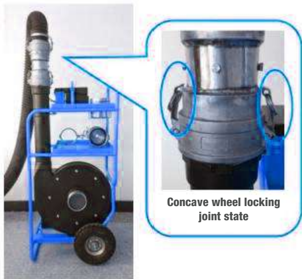
High-flow pipeline positive pressure test; test
