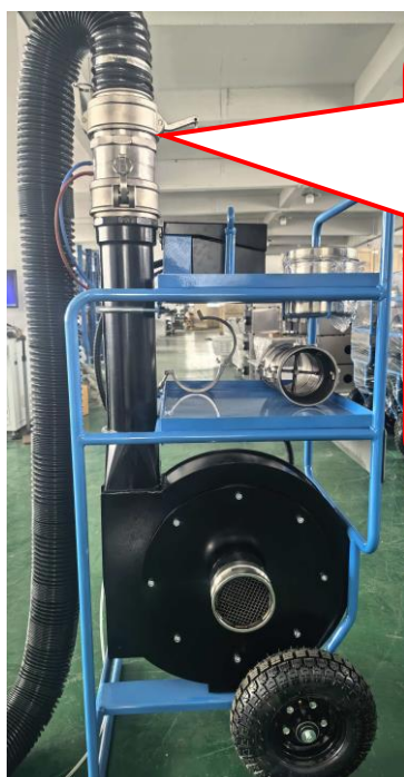
High flow Duct testing under positive pressure
