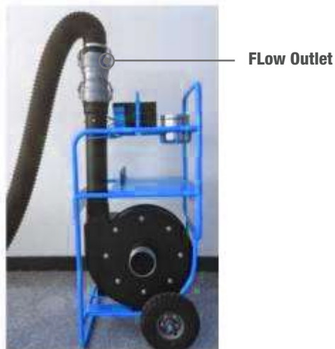
Low-flow duct testing under positive pressure
