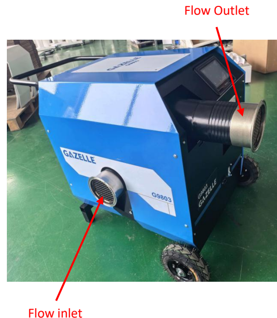
High flow Duct testing under Negative pressure
