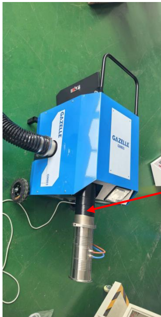
High flow Duct testing under positive pressure
