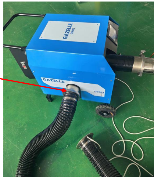
High flow Duct testing under Negative pressure
