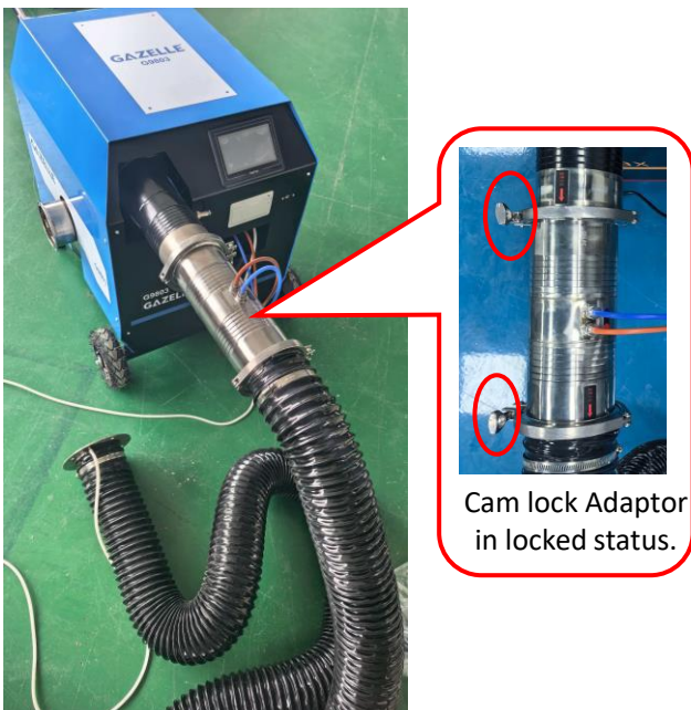
High flow Duct testing under positive pressure
