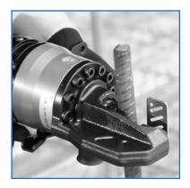
**CUTTING STABILITY**Adjustable stopper holds the rebar at 90° to the cutting blade for more
